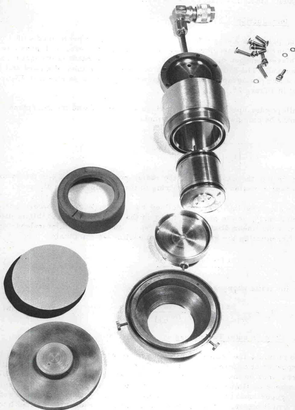
Figure 27 EXPLODED VIEW OF HIGH PRESSURE X-RAY CAMERA
